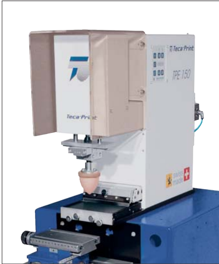
Fig. 1: The pad printing machine TPE 150 is designed for plate sizes from 100 x 100 mm to 150 x 100 mm. Print capacity: 1800 cycles per hour.
