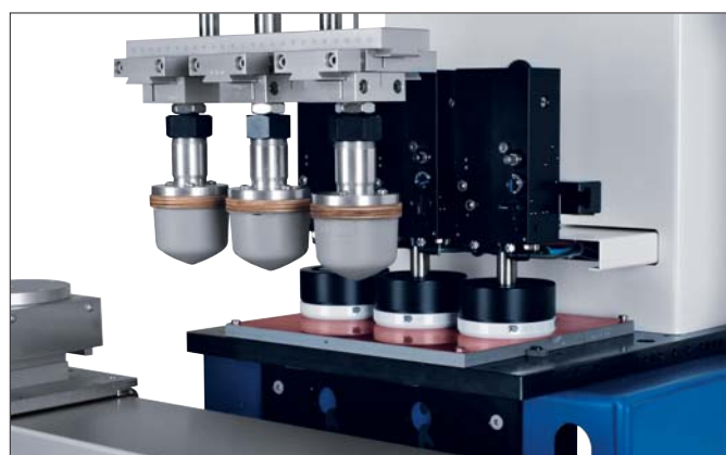
TPE 250 on machine base MS 250 with sliding table VTP, coordinate table KT 30 and angular table
